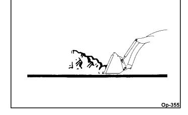
Loaders with 1-lever control, ease lever back toward you to lift and roll back bucket. With series valve, prevent loader stall by not lifting and rolling back at the same time.
